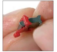
If you removed the plastic part from the pawls, refit it so as the spring clipping pin is in the inside bend radius of the pawl.
