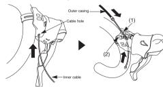
When removing parts in order to replace the inner cable, the work can be carried out more easily if the unit cover is removed as shown in the
