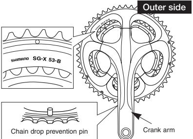
With the marked surface of the smaller chainring facing away from the crank arm, set the chainring so that the △ mark is lined up with the crank arm position.
