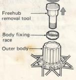
3. When the body fixing race is difficult to remove from the outer body, screw the bolt part of the freehub removal tool into the body fixing race and pull it straight
