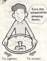
2. Turn the wheel while pressing down. Turn the wheel clockwise to disassemble and counterclockwise to assem-
