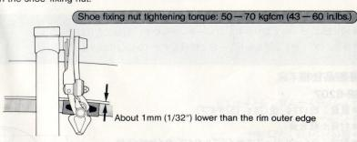
3) To fix the brake cable, set the quick release lever to "CLOSE" position. Connect the cable to the brake lever, pass it through the outer adjusting bolt, catch it between the cable fixing plate and the cable fixing shaft, and tighten up the cable fixing bolt with the 5mm hexagon wrench (TL-WR35)
