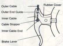
2) Pull the outer cable to take out the cable together with the outer end guide. Now the cable can be removed from the lever grip.
